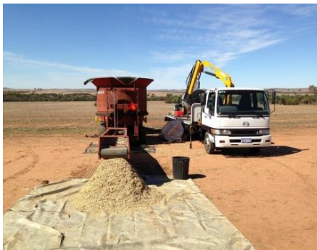
Figures Three, Four, Five (Left to right, above): demonstrate the process used to grind the chipped African Boxthorn material into a finer material for pyrolysis. Figure Six(bottom right) is the before (right) and after (left) photo after material had passed through the tub grinder
