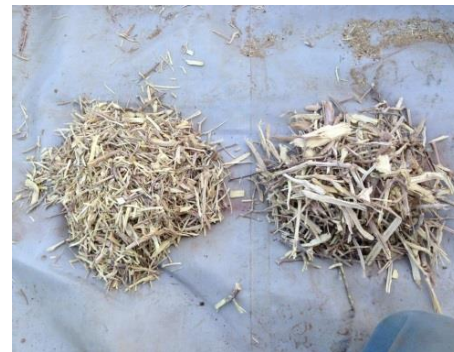
Figures Three, Four, Five (Left to right, above): demonstrate the process used to grind the chipped African Boxthorn material into a finer material for pyrolysis. Figure Six(bottom right) is the before (right) and after (left) photo after material had passed through the tub grinder
